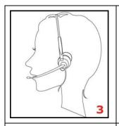
To adjust the headband, lengthen or shorten the adjustment rod until it fits comfortably. The click-stop feature keeps the headband securely adjusted. Position the headset receiver so that the foam cushions sit comfortably over the center of your ears.
