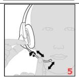
Hold the receiver securely against your ear with one hand. With the other hand, use the boom to adjust the microphone to about one finger distance to your lips.
