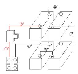
Note: Don't reverse battery polarities, or battery will be damaged
