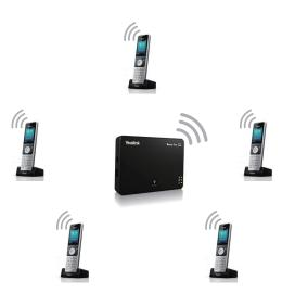
The W56P systems can be expanded up to a total of 5 cordless handsets by adding the W56H or W52H cordless handsets
