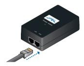
4. Connect the *Power Cord* to the power port on the *PoE Adapter*. Connect the other end of the *Power Cord* to a power source.
