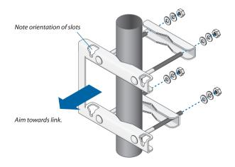
3. Loosen, but do NOT remove the eight *Lock Bolts* located on the *Alignment Bracket*.
