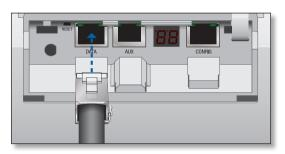
Create a strain relief for the Ethernet cable by feeding a cable tie through the tie slot under the cable. Then wrap the cable tie around the cable and tighten.
