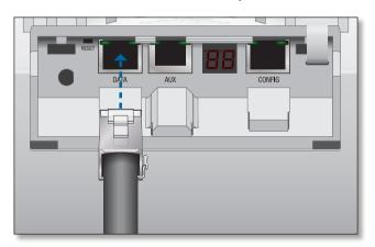
3. Connect the other end of the Ethernet cable from the *DATA* port to the Ethernet port labeled **POE** on the PoE Adapter.
