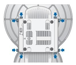
4. Ensure that there is a 6 mm gap between the head of each *M8x14 Serrated Flange Screw* and the *Alignment Bracket*.
