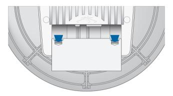
2. Connect an Ethernet cable to the DATA port.
