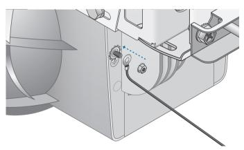
c. Secure the other end of the ground wire to the grounded mast, pole, tower, or grounding bar.
