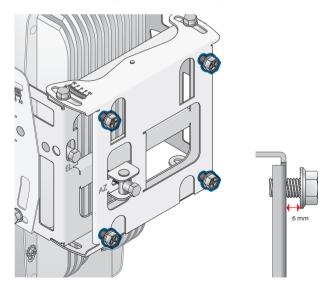
5. Lift the airFiber AF24 and align the four *M8x14 Serrated Flange Screws* with the slots on the *Pole Mount Bracket*. Seat the screws in the slots. Securely tighten the screws.
